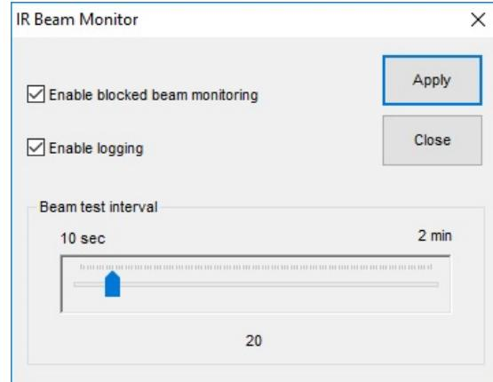
When the beam monitoring is enabled, a message box along with a shaded vertical and/or horizontal bar will pop up to indicate the failed beams or blocked area. Touch will not function within the shaded area on the display until the failed condition is corrected.
