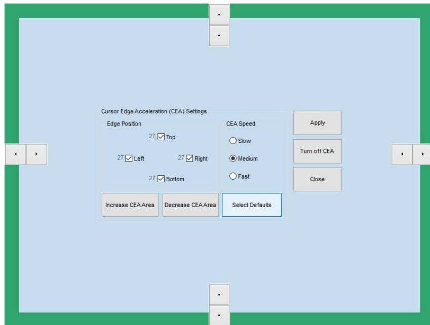
To enable CEA, click on the "Select Default" button and specify the desired parameters. The position of CEA may be manipulated for all edges at once by means of the "Increase/Decrease CEA Area" buttons, or individually by means of the arrows along each edge. Additionally, CEA for edges may be disabled by unchecking their respective box.
