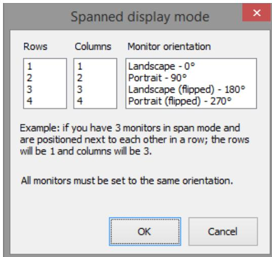
Enabling the “Spanned display mode” option followed by clicking the “Calibrate Touch Screens” button in the main EloConfig page will display a configuration window asking you to provide the number of rows, columns, and monitor orientation in the spanned setup. After
